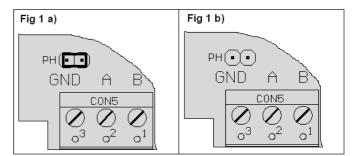
In the case the module is the last on bus, the jumper must be placed according to Fig 1 a) to close the chain BUS. In other situations it should remain as in Fig 1 b).
