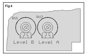
Input sensitivity may be changed turning the potentiometers RV1 and RV2.
