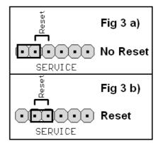
**Reset:** To perform a reset interrupt power to the module 12VDC for a few seconds or place the jumper according to (Fig 3 b) for about 3 seconds to put it back in its original position (Fig. 3 a).
