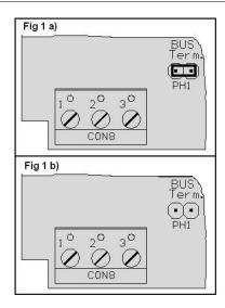
In the case of the module is the last bus on the bus a jumper, according to Fig 1 a), must be placed, to close the chain BUS. In other situations it should remain as in Fig 1 b).
