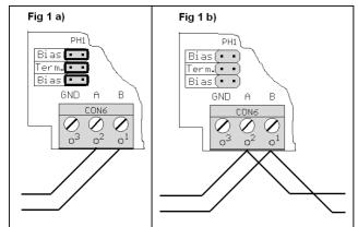
In case the module is the last on the bus Bus, jumpers should be placed according to Fig 1 a) to close the chain BUS.) In case of very large bus length, you may need to put the jumper *Term*. In other situations they should remain as in Fig 1 b).
